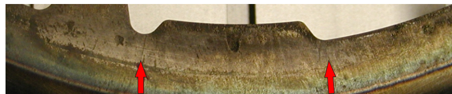
Cracks (red arrows) in an inductively tempered component from the automotive industry
